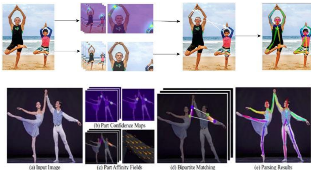
Figure 3. OpenPose steps for estimating human pose.
